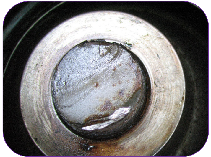
Photo 2: Close-up of the fractured bolt.
