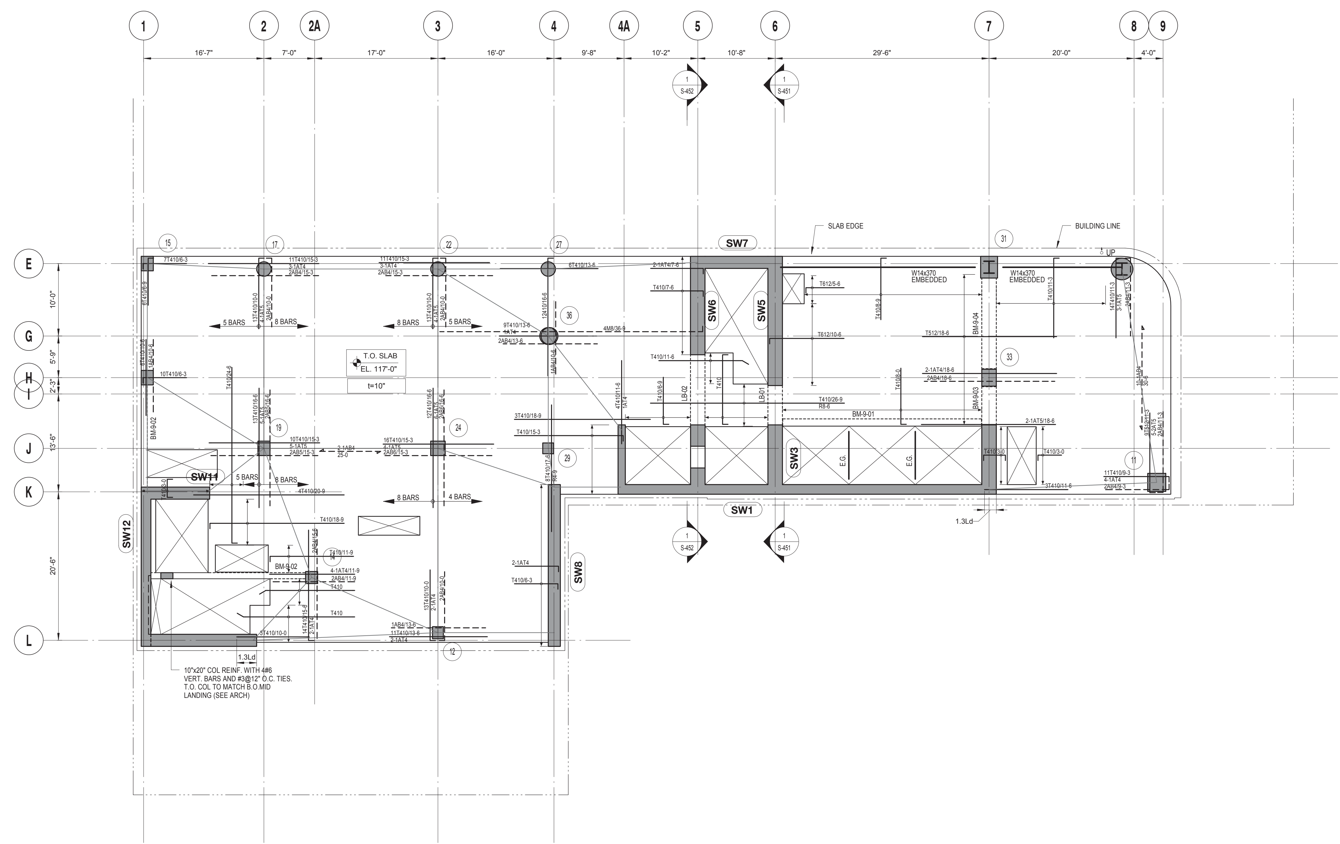
9TH FLOOR REINFORCEMENT PLAN SCALE: 1/8" = 1'-0"
